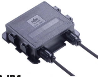
ESP-JB4 4-rail, with diodes, 12A potted/ 10A non-potted, IP67, TUV
